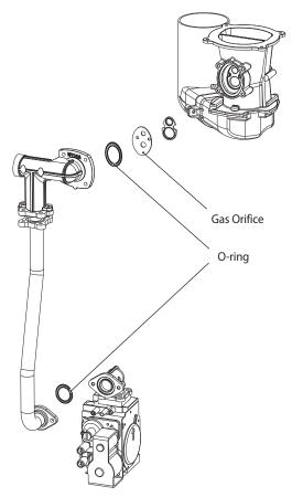
Figure 5. Exploded view of Gas assembly
