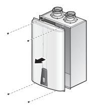
Loosen the screw indicated in the figure below and connect a manometer to the pressure port. Reset the manometer to zero before use.
