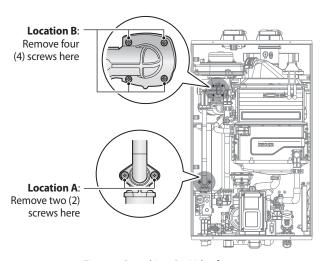
Figure 3. Detaching Gas Valve from Gas Inlet Pipe and Fan Motor Assembly
