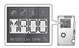
On the slave water heater, press and hold the **Diagnostic** and **Down**(-) buttons for more than 2 seconds. "SL.01" will appear on the display to confirm that this water heater is set as a slave.
