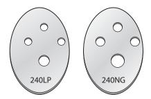
Figure 6. Orifice identification
