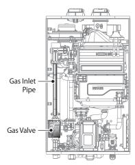
Figure 2. NPE Series Internal Components
