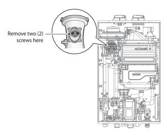
Figure 4. Access to Gas Orifice in Fan Assembly
