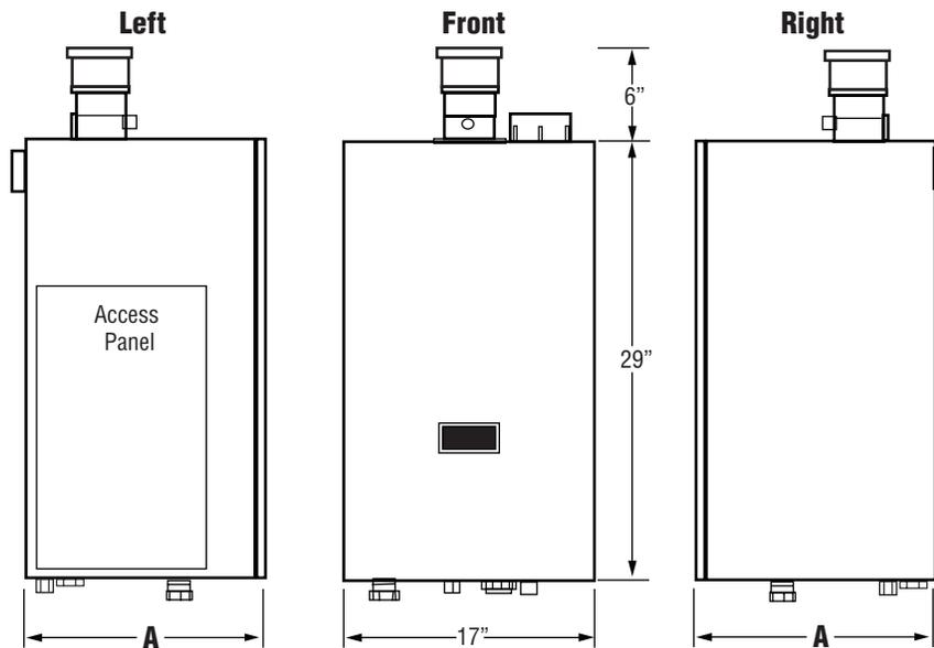
NOTE: Optional combi kit extends 13" below boiler (150 MBH, 180 MBH), with all connections on left side
